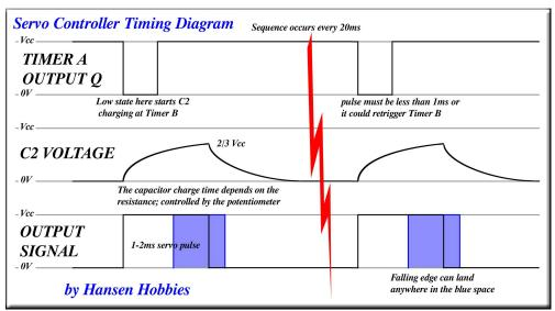
P1 is a 10K $\Omega$  potentiometer that can be anything from 0 to 10K $\Omega$ . When you plug in values of 0–10K $\Omega$ , 10K $\Omega$ , and 0.1uF for P1, R3, and C2, respectively, we get results of .001 through .002, exactly the 1–2ms needed for the PWM.
